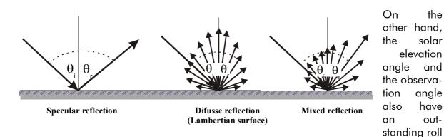
Fig. 4-8: Diverse reflection types according to roughness-surface.
