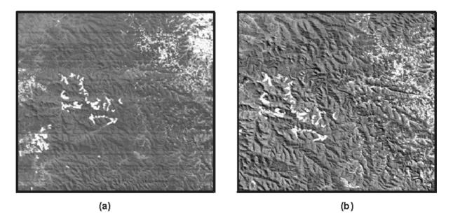
Fig. 4-13: Correction of striping in band 3 Landsat 5 TM image of 1986 a) Original image. (b) Image radiometrically corrected.
