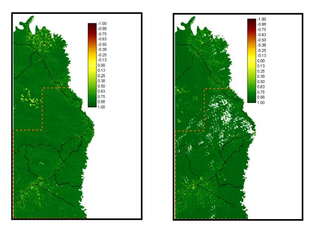
**Fig. 4-26:** NDVI image from 1986 Landsat 5 TM imagery (left) and 2001 Landsat 7 ETM+ (right). The NDVI values range from -1 (dark brown) to 1 (dark green). Demarcated area corresponds to study area.
