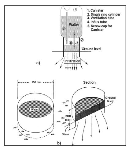
Fig. 5-17: Single ring infiltrometer (a and b).
