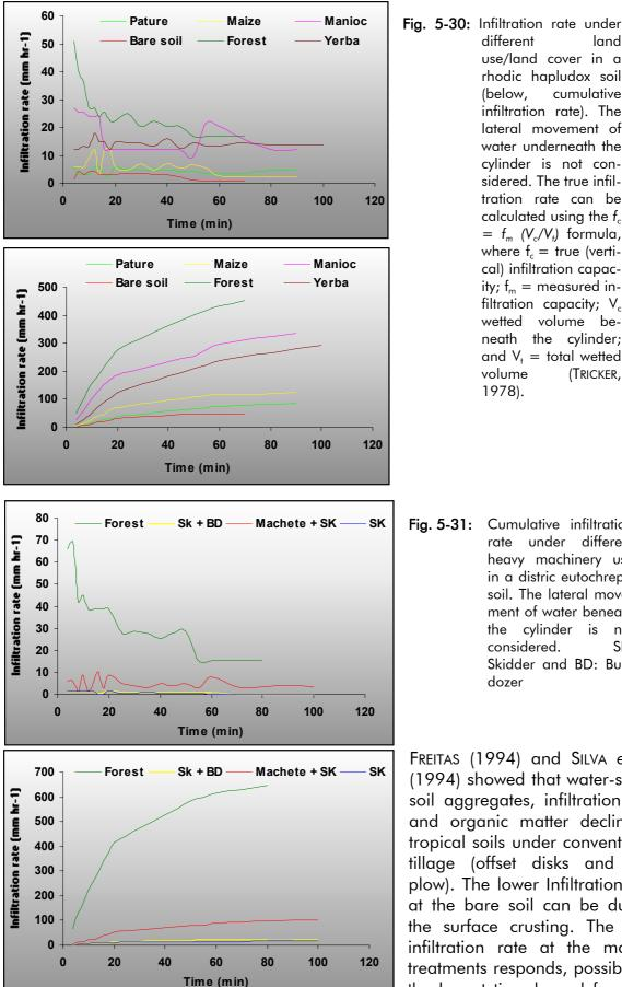
different land use/land cover in a rhodic hapludox soil (below, cumulative infiltration rate). The lateral movement of water underneath the cylinder is not considered. The true infiltration rate can be calculated using the  $f_{\rm c}$  $= f_m (V_c/V_t)$  formula, where  $f_c = true$  (vertical) infiltration capacity; f<sub>m</sub> = measured infiltration capacity;  $V_{c}$ wetted volume beneath the cylinder; and  $V_t = total$  wetted volume (TRICKER, 1978).
