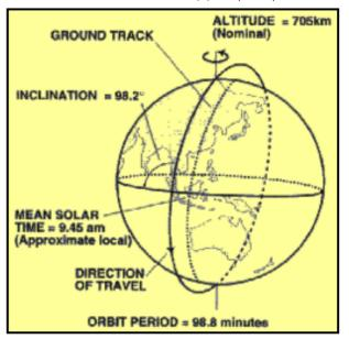
Fig. 4-10: Landsat's orbit characteristics.
