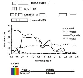
Fig. 4-6: Spectral reflectance characteristics of common earth surface materials in the visible and near-to mid infrared range. The positions of spectral bands for common remote sensing instruments are indicated (Source: RICHARDS, 1999, modified).
