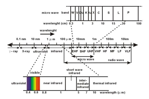
**Fig. 4-5**: Electromagnetic spectrum in the wavelength-range between 0.1nm and 10 km. The relevant spectral range for optical remote sensing is from 0.4 to approx. 2.5 μm.
