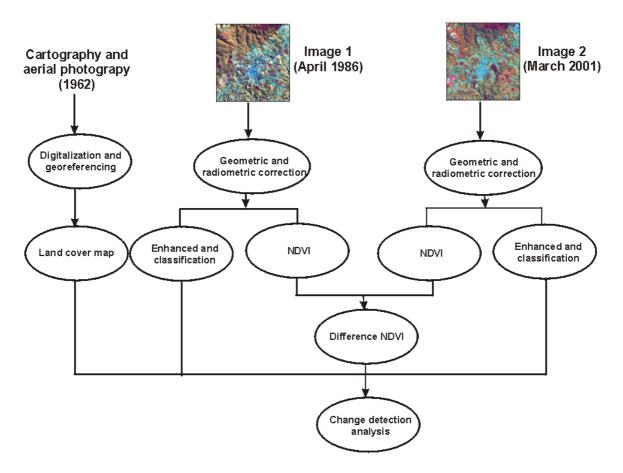
Fig. 4-12: Diagram of land use/land covers change detection based on multitemporal analysis.
