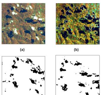
Fig. 4-14: Cloud and shadow masks derived from and applied to a portion of an ETM+ image. a) Original Band 453 (RGB) Image. b) Masked Band 453 (RGB) Image. c) Cloud Mask. d) Shadow Mask.
