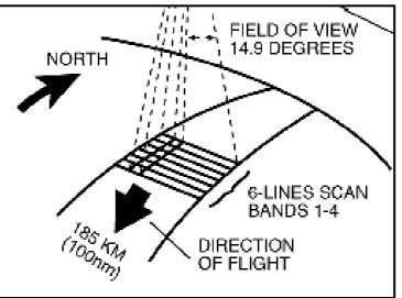
The Landsat 5 has a revisit frequency each 16 days. To be Fig. 4-9: Scanning of the Landsat TM sensor.
