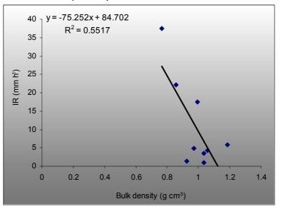
Fig. 5-32: Variation of the infiltration rate according to increase of the bulk density.
