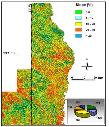
Fig. 5-22: Slope steepness calculated from DGM.
